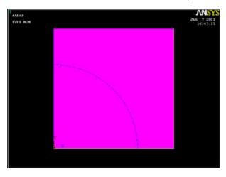
In the *Input* window, ANSYS now tells you to "pick or enter areas to be subtracted". So select the circular sector by holding down and releasing the left mouse button. Click *OK*.
