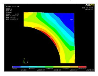
The two results compare well with the finer mesh contours being smoother as expected. Compare the maximum stress and displacement values:
