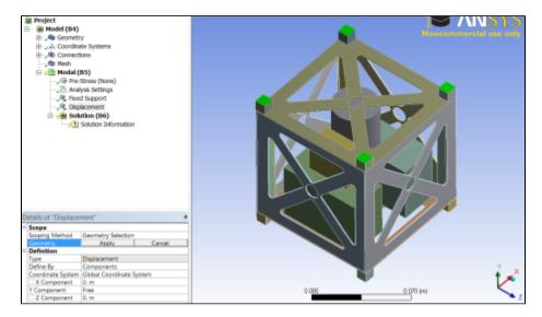
To simulate the constraint of the side rails, set the X and Y components to Constant (0 m) and the Y component to Free.
