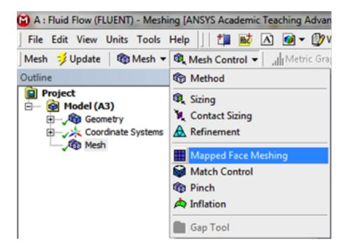
Now, the *Mapped Face Meshing* still must be applied to the pipe geometry. In order to do so, first click on the pipe body which should then highlight green. Next, *(Click) Apply* in the *Details of Mapped Face Meshing* table, as shown below.
