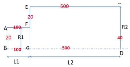
In this section the geometry will be meshed. The cell numbers on the edges of the desired mesh are shown here:
