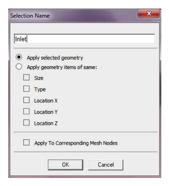
Now, create named selections for the remaining edges and name them according to the diagram. Since the "Centerline" consists of two edges thus when naming the centerline you should use "Ctrl" to select both parts. For the "Wall", use "Ctrl" to select three edges.
