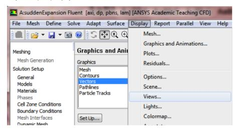
Under *Mirror Planes*, only the *axis* (or centerline) surface is listed since that is the only symmetry boundary in the present case. Select *axis* (or centerline) and click *Apply*, as shown below.
