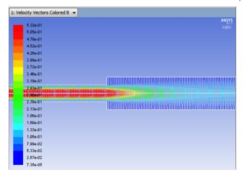
The velocity vectors provide a picture of how the flow develops downstream from the inlet and redevelops from the expansion entrance.
