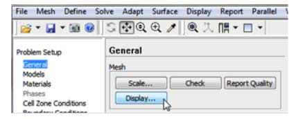
The previous step should cause the *Mesh Display* window to open, as shown below. Note that the *Named Selections* created in the meshing steps now appear.
