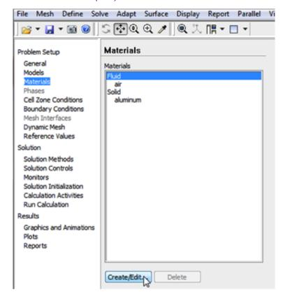
In the Create/Edit Materials menu set the Density to 1kg/m^3 (constant) and set the Viscosity to 3.61e-2 kg/(ms) (constant) as shown in the image below.
