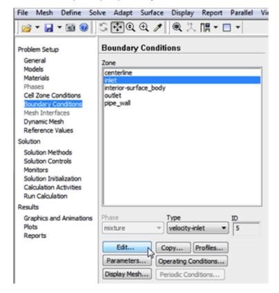
Note that the **Boundary Condition Type** should have been automatically set to **velocity-inlet**. Now, the velocity at the **inlet** will be specified. In the **Velocit Inlet** menu set the **Velocity Specification Method** to **Magnitude**, **Normal to Boundary**, and set the **Velocity Magnitude** (**m/s**) to 0.277 m/s, as shown below.
