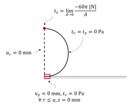
Along the frictionless contact interface, we specify the following boundary conditions.
