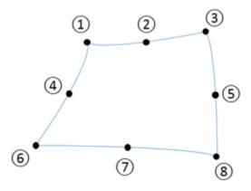
Each of the eight nodes shown above can be described by displacement vectors (translational and rotational components, depending on the element type) and by force vectors. Finite element method first solves for the nodal displacement field with the specified boundary conditions. The underlying system of equations that ANSYS solves for is shown below.
