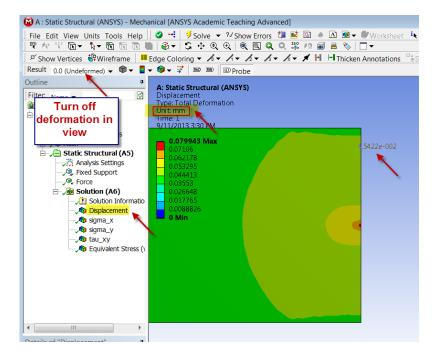
I get a value around 0.045 mm at the right end away from the point load. This is about a 10% deviation from the hand calculation result of 0.05 mm we obtained in our *Pre-Analysis*. This is a reasonable agreement considering that the hand calculation ignores the high stress areas at the left and right ends. But these high stress areas (both tensile and compressive) affect relatively small areas of the model and so don't contribute a lot to the overall displacement.
