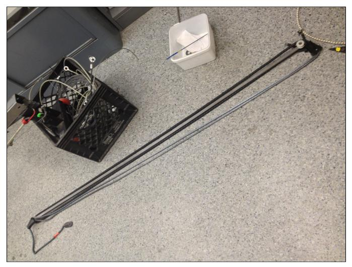
Because the chain wraps around a sprocket-pulley, it's as if there are two chains running right next to each other, in opposite directions. We made sure the chains didn't criss-cross in order to make sure the chain runs smoothly, noiselessly, and without wear-and-tear.
