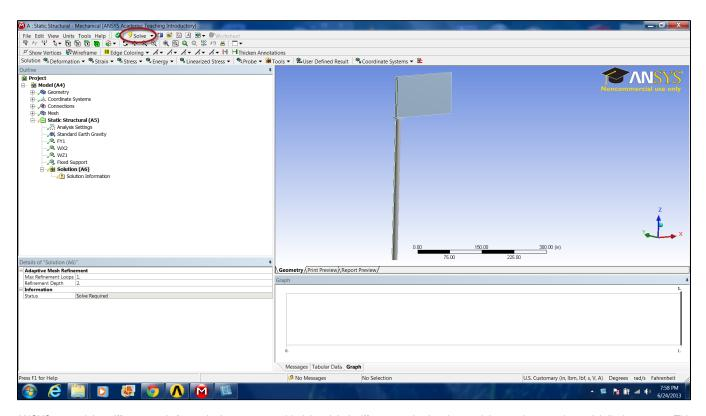
ANSYS created the stiffness matrix for each element, assembled the global stiffness matrix, then inverted the matrix to get the nodal displacements. This is the bulk of the computation that ANSYS performs. The following results are derived from these nodal displacements.
