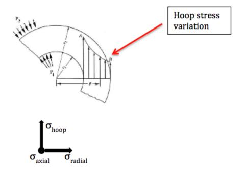
By using the parameters given in the problem statement and the above formulae for hoop stress, we find that the maximum hoop stresses using the thin-wall and thick-wall approximations yield 3000 psi and 3571 psi, respectively. This corresponds to a 16% difference which tells us that the thin wall theory might not be adequate for this geometry. Thin-wall theory actually gives good results when b/a ratio is less than 1.10, and that is not the case here.
