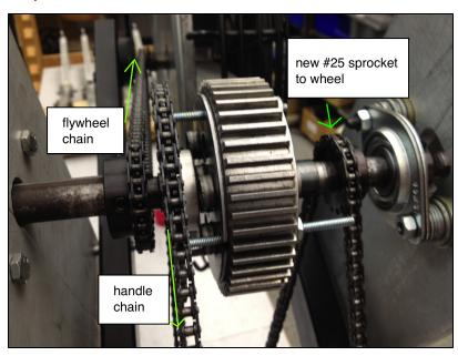
The wheel axle looks the same, but with different sized chain+sprocket that connects the differential to the wheel. Everything on the wheel axle spins with the same angular velocity; nothing rotates freely or independently of the axle.
