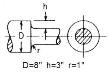
The pressure load P/A on the smaller cross-section is 1000 psi.
