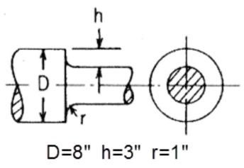
The pressure load P/A on the smaller cross-section is 1000 psi.
