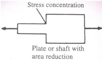
So the problem becomes amenable, let's consider a relatively small fillet placed at the step to reduce the stress concentration to a finite value.
