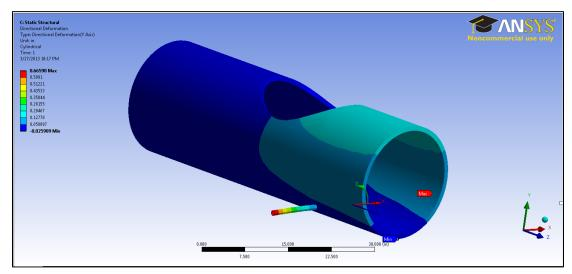
The maximum tangential deformation occurs at the tip of the suspension links, which is reasonable, and the tangential value is 0.0226 inches.
