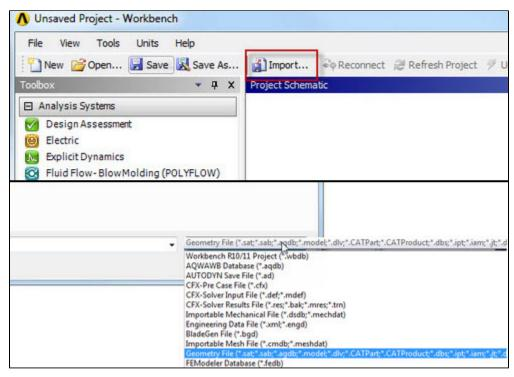
Once we are satisfied with our geometry, we can close the design modeler. Now, we should be looking at the *Project* window. To connect the geometry to the project, click and drag . As soon as you drag the box, ANSYS will highlight the geometry and model boxes in the main project.
