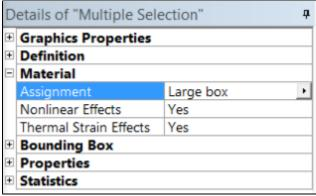
Now assign the small box material to "Small Box 1" and the cylinder material to "Cylinder". The internal components will now simulate a more realistic mass rather than a solid piece of aluminum.
