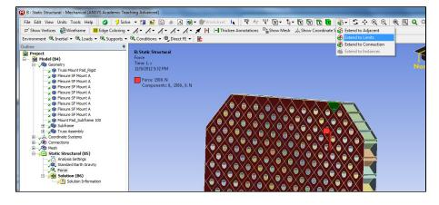
Using the Components definition, create 1500N in the positive Y direction.
