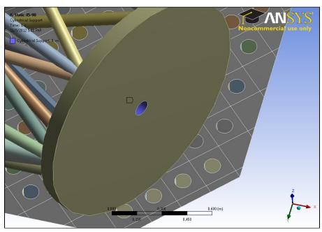
We don't want to over-constrain it, so make sure only the Tangential definition is fixed, letting the Radial and Axial movements be free.
