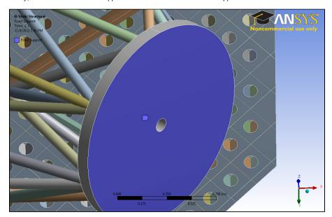
While this fixes one direction of motion, it does not prevent the base pad from translational movement parallel to its plane. To constrain this, we create a Cylindrical Fixed Support and apply it to the middle hole.
