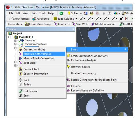
For this contact, you will want to select the four faces of the shell geometry (Face Sheet Surface\_100mm holes) and apply it as the Target body (Red). Then select the flexure mount surface near it and apply it as the contact bodies (blue). You should be able to select it through the shell model.
