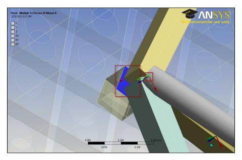
Do this for the remaining flexure mounts, and the center submount. There should be a total of 9 Joints created from this.
