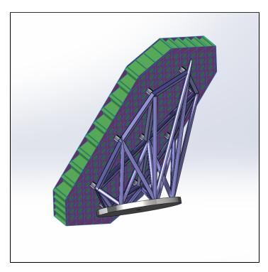
This Telescope Truss will contain mirrors on the frame, (not modeled), and can be rotated with the Telescope, meaning that its orientation with respect to gravity is variable.
