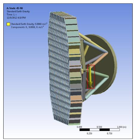
Now, we wonder about the simplifications we can make in the model. We notice that the truss bars can be modeled as beams, and so we will replace the solid geometries with line bodies with a cross-sectional area. This will reduce and simplify the model, decreasing the computational time while keeping the same validity.
