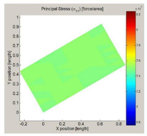
We again get a homogeneous state of stress as expected. From the colorbar, the stress value is around 75 MPa which matches the applies normal traction. Click on *Plot* in the *Export* menu and save the plot as sigma\_11.fig.
