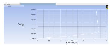
Then, return to the Solution XY Plot menu and select both line1 and outlet under Surfaces. Next, click Plot and you should obtain the following figure.
