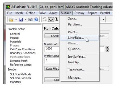
We'll create a straight vertical line from (x0,y0)=(0.5,0) to (x1,y1)=(0.5,0.5). Select *Line Tool* under *Options*. Enter x0=0.5, y0=0,x1=0.5, y1=0.5. Enter line1 under *New Surface Name*. Your *Line/Rake Surface* menu should look exactly like the following image.
