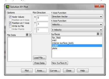
Now, click *Plot*. The plot of the x component of the velocity as a function of distance along the *outlet* now appears.
