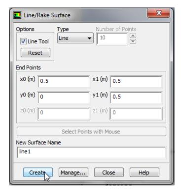
Next, click *Create*. Now, that the vertical line has been created we can proceed to the plotting. Click on *Plots*, then double click *XY Plot* to open the *Solution XY Plot* menu. In the *Solution XY Plot* menu, use the settings that were used from the section above, except select *line1* under *Surfaces* and deselect any other geometry sections. Make sure that *Write to File* is not selected, then click *Plot*. You should obtain the following output.
