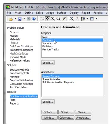
In the Contours menu, set Contours of to Pressure... and set the box below to Pressure Coefficient. Next, select Filled and set Levels to 90. Your Con tours menu should look exactly like the following image.
