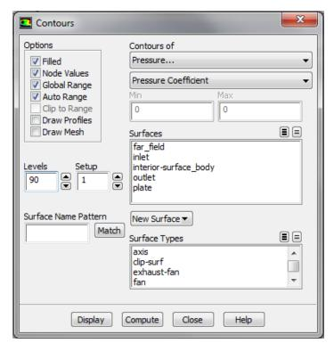
Lastly, click *Display* in the *Contours* menu to generate the contour plot. You should obtain the following output.
