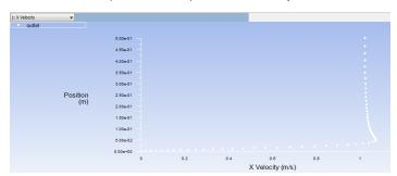
In order to increase the legibility of the graph, we will plot the data as a line rather than points. To turn on the line feature, click on *Curves...* in the *Solution XY Plot* menu. Then, set *Pattern* to ----, set the *Weight* to 2 and select nothing for *Symbol*, as shown below.
