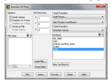
Make sure that for both the x and y axes, that *Auto Range* is selected. Remember, that you must click *Apply* to implement the changes you make. Then, click *Plot* in the *Solution XY Plot* menu and you should obtain the following output.
