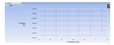
It is of interest to compare the numerical velocity profile to the velocity profile obtained from the Blasius solution. In order to plot the theoretical results, first click here to download the necessary file. Save the file to your working directory. Next, go to the *Solution XY Plot* menu and click *Load File...* and select the file that you just downloaded, *BlasiusU.xy*. Lastly, click *Plot* in the *Solution XY Plot* menu. You should then obtain the following figure.
