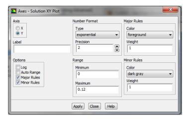
Then, click Apply in the Axes - Solution XY Plot menu. Now, select X for Axis and select Major Rules and Minor Rules, as shown below.
