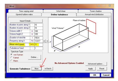
To replace the default wind file with the user-defined wind file, click on the *Time varying wind* tab. Use the browse button to locate the file you have generated and replace the default wind file (demo\_a.wnd).
