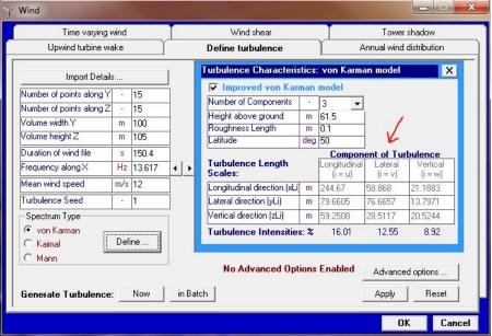
With limited options, we will create a turbulent wind with a different mean wind speed while leaving everything else unchanged. Change the mean wind speed to 11 m/s. Click on the Now button next to Generate Turbulence. You will be prompted two dialogues and you may click on OK to proceed. Save the wind file in the desired directory.
