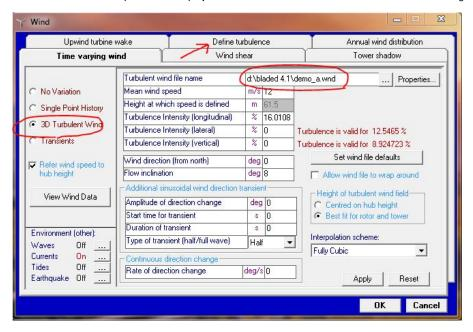
The default wind in the demo uses a pre-defined turbulent wind file called **demo\_a.wnd** and this file is stored in the Bladed directory. We can define a new turbulence wind file in the **Define turbulence** tab, indicated by the arrow.
