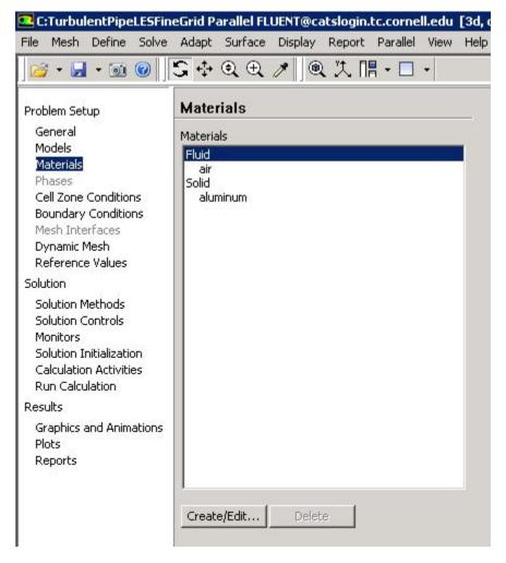
In the Create/Edit Materials menu set the Density to 1.331 kg/m^3 (constant) and set the Viscosity to 2.34e-05 kg/(ms) (constant) as shown in the image below.
