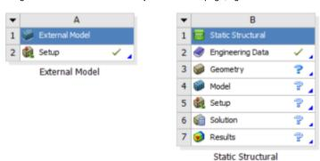
In the Project Schematic page, click and drag Setup from External Model and drop it onto Model in Static Structural.
