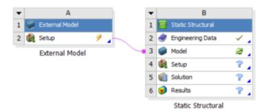
This will load the External Model into ANSYS Mechanical. When External Model is linked with *Model* in *Static Structural*, the geometry and mesh in the External Model is transferred to Mechanical and the user can proceed straight to setting up the physics.
