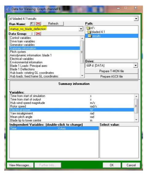
Click on Channel 2 and change the path to the desktop to find "demo\_steady\_wind\_11". Make sure "demo\_steady\_wind\_11" appears under *Run Name*. S elect summary information and electrical power, as shown in the previous step.
