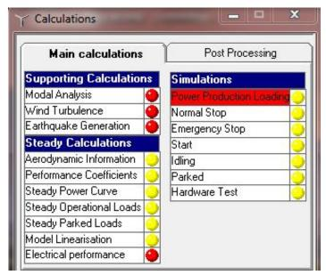
The red circles next to each calculation and simulation in the calculation window indicate none of the required input parameters are defined. The yellow circle indicates that only a part of the required inputs are defined for a given simulation. Green circle indicates all the inputs are fully defined and the simulation is ready to be carried out.
