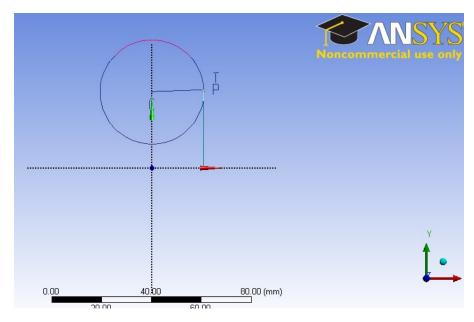
Use the *General* dimension tool to create dimensions for the line and the radius of the arc. The length of the line is 30 mm and the radius of the arc is 25 mm. Your sketch should look like this:
