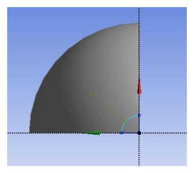
Click on the Extrude icon and select the quarter circle for the geometry. In the Details of Extrude1 window, set the Depth to 15 mm.
