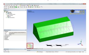
Now, while pressing CTRL, click hover over the different layer options until you have identified the surface you wish to select (in this case, a surface on the electronic board); click on that layer. Then, while still holding down CTRL, click the top layer to unselect the top surface. Repeat this process for the ten vertical chips and the battery. When you have finished selecting the surfaces, right click, and create a named selection and name it, HeatGeneration.
