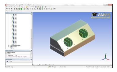
Once you are sure you have the correct geometry, right click **Solid** and select **Suppress All Other Bodies**. This should leave only the fill geometry and the chips visible.
