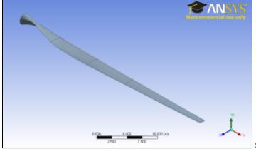
Click here to enlarge imageThe blade is composed of an outer surface and an inner spar. The spar is 0.02 meters thick and the outer surface is of varying thickness. A table containing the material properties of the two parts is below. Structural steel will be used for both the blade and the spar.
