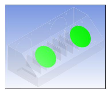
When the two surfaces have been selected, right click and select *Create Named Selection*. Name the selection, Inlet. Repeat the process for the two holes corresponding to the outlet, and name the selection, Outlet.
