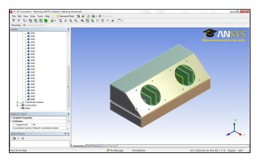
Once you are sure you have the correct geometry, right click **Solid** and select **Suppress All Other Bodies**. This should leave only the fill geometry and the chips visible.
