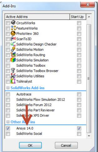
After ensuring ANSYS Add-in is activated, the user can load the Solidworks model into ANSYS by clicking on "Workbench" from "ANSYS 14.0" from the menu tool bar.
