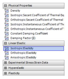
In the Properties of Outline Row 4: Cornellium window, Set the Elastic Modulus units to psi, set the magnitude as 29e6, and set the Poisson's Ratio to .3.
