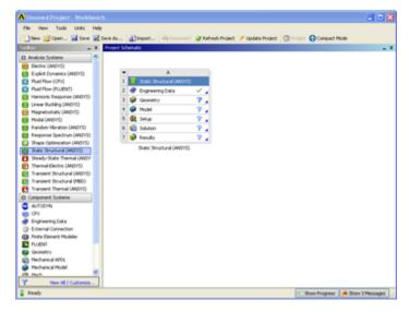
Name the Project "Plate with a Hole" by double clicking the text Static Structural and typing in Plate with a Hole.
