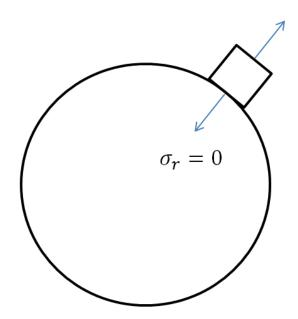
We see that Sigma-r at the hole is the normal stress at the hole. Since the hole is a free surface, this has to be zero.
