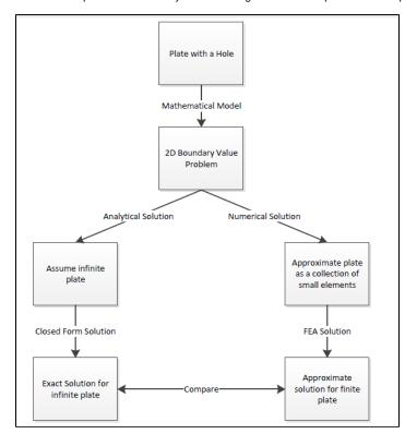
Let's first review the analytical results for the infinite plate. We'll then use these results to check the numerical solution from ANSYS.
