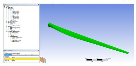
Select function from the drop down list in *Thickness*. Enter the thickness as a function of length: 0.03-0.00048485\*x. The thickness graphics will be
