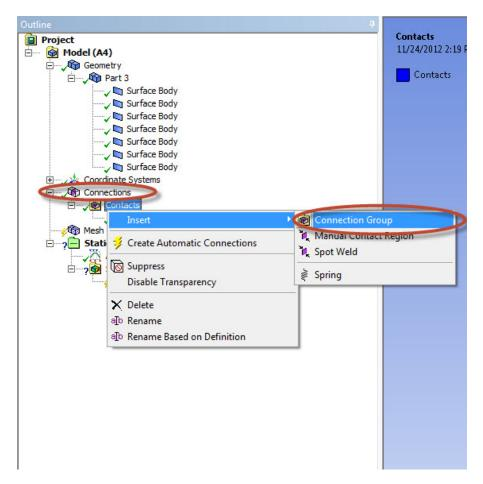
In the connection group named Contacts 2, change the Face/Face detection to No and Face/Edge detection to Yes.
