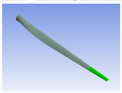
When the surface have been selected, press *Geometry > Apply* in the *Details* window. Next, select *Define By > Components*. Define the *Y Component* as -1000 N.
