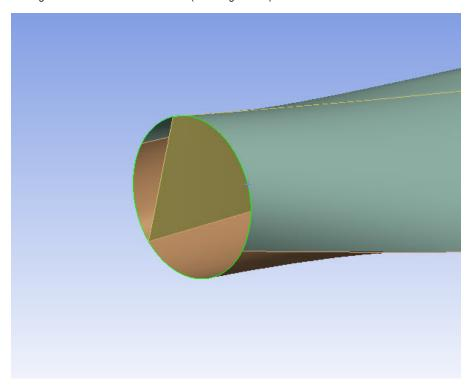
When both edges have been selected, press *Geometry > Apply*.
