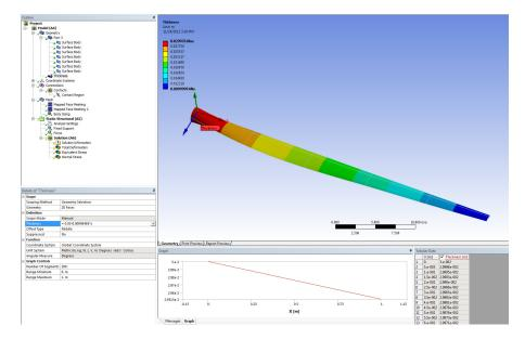
The thickness of the spar is 0.02 meters. Locate the appropriate surface bodies that represent the spar and change the thickness to 0.02 meters.
