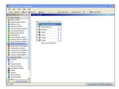
Name the Project Wind Turbine Blade by doubling clicking Static Structural (ANSYS) underneath the project schematic.
