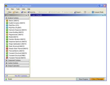
To begin, we need to tell ANSYS what kind of simulation we are doing. If you look to the left of the start up window, you will see the Toolbox Window. Take a look through the different selections. Because we are only doing a force loading, we will be doing a Static Structural simulation. Load the Static Structural tool box by dragging and dropping it into the Project Schematic.
