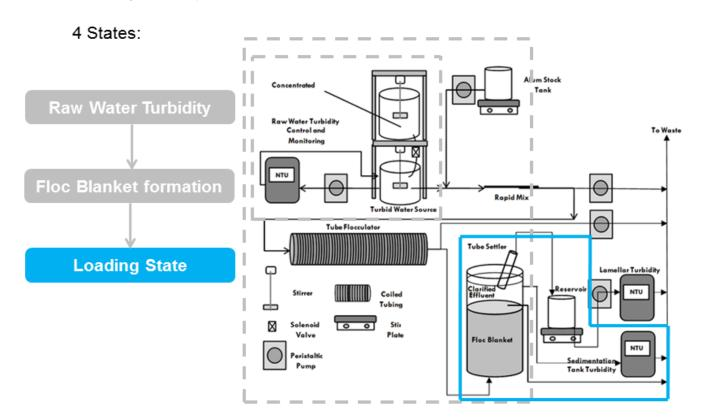
In the "Withdrawal State", once the floc blanket reaches the height of the floc weir, the effluent turbidity in the tube settler is sampled. For small experimental flow rates, a reservoir is used to accumulate and then sample effluent turbidity. Turbidity data is acquired and recorded every 5 seconds from the turbidimeters. After the task is accomplished the setup then re-enters the "Loading State" and keeps going back-and-forth between the two.
