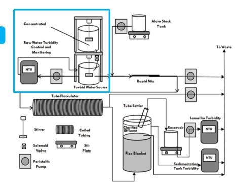
In the "Floc Blanket formation" stage, the raw water turbidity is combined with the alum solution – dosage of 45 mg/L (4.23 mg/L Al) was utilized. Here we used the flow rate of 712.6 mL/min throughout all experiments. The solution of raw water and alum were rapidly mixed by flowing through a tube 4.8 mm ID (inner diameter), 1 m in length with an energy dissipation rate of 0.1 W/kg.
