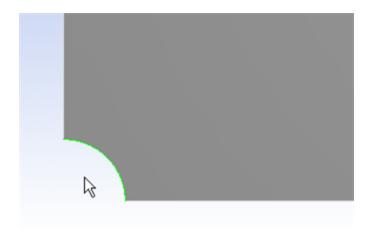
In the details window, change the Refinement parameter from 1 to 3, this will give us the finest mesh at the hole which will improve accuracy of the simulation.
