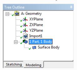
Specifically, there should be a *1 Part, 1 Body* expandable tab. Expand the tab and the only contents should be *Surface Body*. In certain versions of ANSYS, it has been reported that superfluous line bodies are being imported as well. If you see the line bodies in this window, right click each of the line bodies and select *Supress*. The line bodies will cause errors when we are meshing the body.
