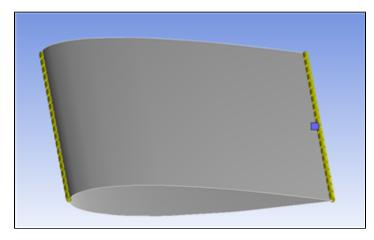
Again, in the *Details* window change the settings such that *Type > Number of Divisions* and *Behavior > Hard*. This time, change the *Number of Divisions* to 20. Generate the mesh by selecting **Mesh > Generate Mesh**.
