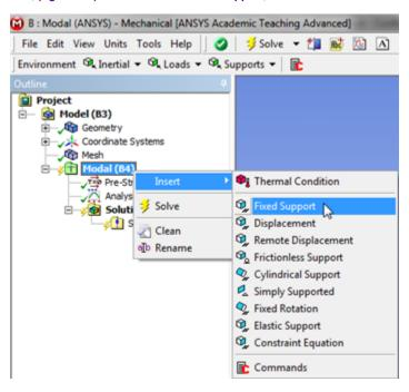
Next, click the *vertex selection filter* button, . Then, click on the left end of the beam and apply it as the *Geometry* in the "Details of Fixed Support" table
