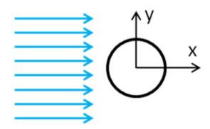
Consider the steady state case of a fluid flowing past a cylinder, as illustrated above. Obtain the velocity and pressure distributions when the Reynolds number is chosen to be 20. In order to simplify the computation, the diameter of the cylinder is set to 1 m, the x component of the velocity is set to 1 m/s and the density of the fluid is set to 1 kg/m^3. Thus, the dynamic viscosity must be set to 0.05 kg/m\*s in order to obtain the desired Reynolds number.
