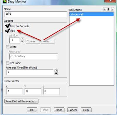
Then check Print to Console and Plot. Next, click cylinderwall, which is located under Wall Zones. Lastly, click ok
