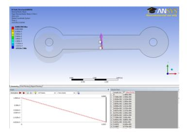
While the strain along the entire strain gauge is useful, what we really want is the average along the strain gauge. Right click anywhere in tabular data window, and go to **Export**. Save the file as an .xls file and name it **Strain data**. Open the file, and average the data by selecting all of the strain data, then going to *Formulas > AutoSum > Average*. At the bottom of the data, we will see the calculated average of the strain gauge: 4.5167E-5 in/in.
