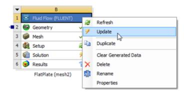
Now, wait a few minutes for FLUENT to obtain the solution for the refined mesh. After FLUENT obtains the solution, save your project.
