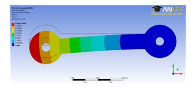
From the deformed view, we can see that the crank deformed basically as we would expect from this loading.
