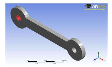
Next, we need to specify the magnitude of the force. We want the 100 lb force to point in the negative y-direction. To do this, we need to select *Define By* > *Components*, then specify the *Y Component* of the force to be -100 lbs.
