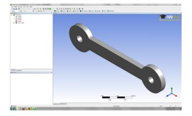
Now that we have verified we are using the geometry we want, we need to tell ANSYS that this is the geometry we want to use. Close the Design Modeler
