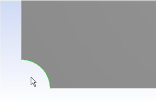
In the details window, change the Refinement parameter from 1 to 3, this will give us the finest mesh at the hole which will improve accuracy of the simulation.
