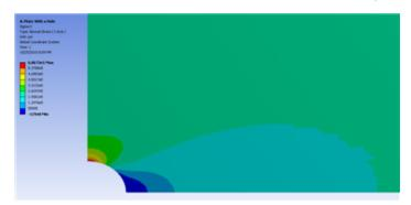
From this, you can see that most of the plate is in constant stress, and there is a stress concentration around the hole. The more red areas correspond to a high, tensile (positive) stress and the bluer areas correspond to areas of compressive (negative) stress. Let's use the probe tool to compare the ANSYS simulation to what we expected from calculation. In the menu bar, click the Probe button; this will display the Sigma-x values at the cursor location as you
