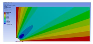
In our pre-analysis, we determined that at r = a the shear stress should be 0 psi. Using our probe tool, we find that the stress ranges between -5 and -500 psi at the hole. Because 500 psi is .05% of the average stress, we can say this result does represent what we expect to happen very well.
