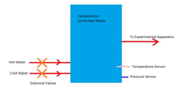
Figure 2: Foam Filtration Raw Water Supply System
