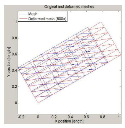
We see that elements have been stretched in the x' direction which is the direction along which the tension has been applied. The elements have also shrunk in the y' direction. This behavior is as expected.
