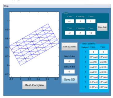
This completes mesh creation. Click on *Mesh Complete*. This puts us back in the main *redAnTS* GUI. We see under *Current Settings* that *rect\_mesh.dat* is the mesh file we are working with. To plot the mesh in this GUI, click on the drop-down menu under *Plotting* and select *Mesh*.
